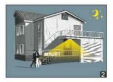
With insufficient daylight, when motion detected.light ON.
